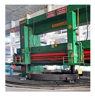
Figure 1. 18-meter turning lathe at the Yongsong Machine Complex.
